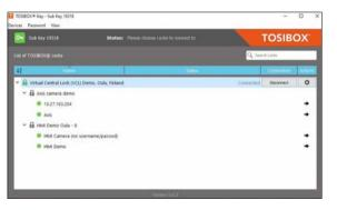
Key user interface (installed from the Key device). In the image you can see TOSIBOX<sup>®</sup> Lock devices which are matched with the TOSIBOX<sup>®</sup> Key and the network devices connected to each TOSIBOX<sup>®</sup> Lock.
